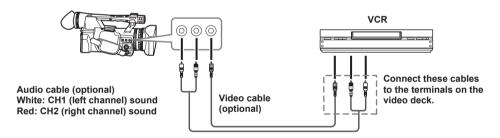
■ When outputting video and audio signals from the camera to an external device, connect to the input terminals of the external device.
