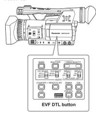
Press EVF DTL button again to return to the original display. "EVF DTL OFF" appears on the screen for about 2 seconds.
