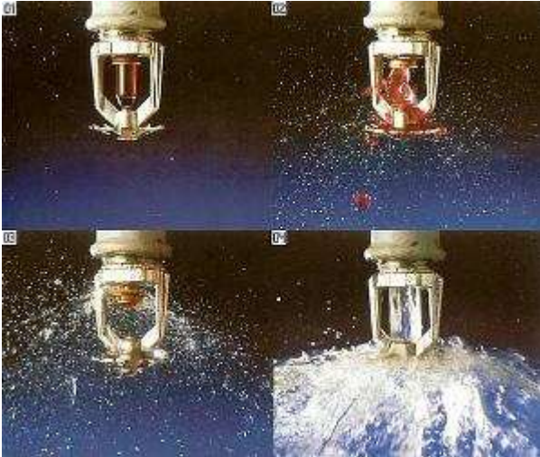
Illustration of a fire sprinkler activated
